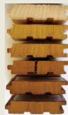
Colour darkens as the temperature in the process is increased
